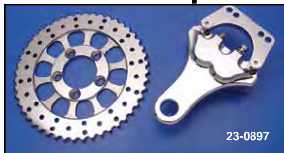
Right Side Billet Rear Caliper Kit fits 1986-99 Softail with integral side mount tail lamp/caliper bracket. Order curved tail lamp separately. VT No. 22-0762
