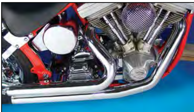
30-0318 shown with full coverage heat shields.
