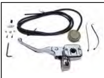
Hydraulic Clutch Handle Kit. Fits 1987-2006 VT No. 26-0996
