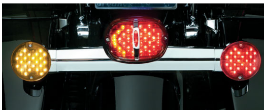
Selected Turn Signal Flashes Amber & Amber Arrow Flashes On Appropriate Side Of Taillight. Other Turn Signal Remains Illuminated Red
