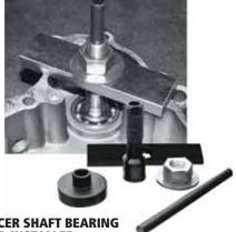
JIMS® BALANCER SHAFT BEARING REMOVER AND INSTALLER
