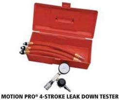
Designed to check percentage of cylinder leakage in a 4-Stroke engine. Can pressurize the cylinder with 60 psi of air with one air source of 70 to 160 psi. The gauge will register the total leakage past the rings, head gasket, intake and exhaust valves.
