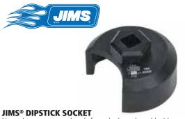
Not only protects your hands from the heat, but aids riders with limited hand strength in easily checking their oil level. Allows riders and mechanics to quickly and safely remove the engine oil level dipstick that lies precariously close to a scorching hot exhaust pipe. Features include a square hole for 3/8 in. ratchet fitment, 7/8 in. hex for wrench fitment and a cutout for clearance around the exhaust pipe.
