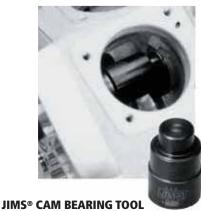
Use to install inner cam bearing.
