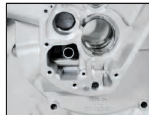
Relocated oil scavenger pick-up reduces oil carry-over by increasing oil scavenge efficiency.
