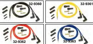
Accel Thundersport 5mm Ignition Wire features half the diameter of stock wire and is extremely flexible. Easy to run through cylinder heads, rocker covers and frame tubes for a hidden look. Packaged with two 5 foot leads, coil ends and 90° spark plug end. Coil end must be terminated. These wires are a 5 mm high gloss silicone wire that is rated for over 550° F and 150 ohms per foot.
