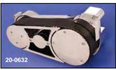
**BDL TF-1000 and TF-2000 "Top Fuel" Street Belt Drives for 1991-up FXST.** Features 14mm by 3%" wide belt, Kevlar Nine (9) Plate Clutch with eleven (11) steels, special pressure plate that uses nine (9) springs for varying spring pressure. Drive includes pulleys, belt, clutch pack, starter jack shaft, inner motor plate with oil filter mount pulley domes and side guard. Polished finish. The TF-2000 features out board bearing support and polished finish.
