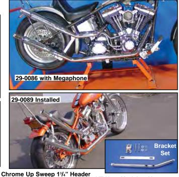
**Chrome Up Sweep 1**<sup>3</sup>/<sub>4</sub>" **Header Sets** will accept straight fishtail extensions or mufflers which must be purchased and mounted separately for Softail or Rigid frames.
