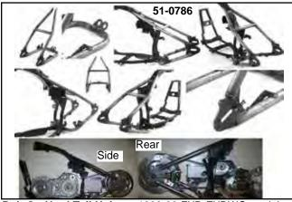
**Bolt On Hard Tail Units** to 1990-98 FXD-FXDWG models. Use stock rear wheel or fit up to 200mm width. Order battery box separately. Bottom attaches to swingarm pivot point to aid in alignment.
