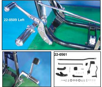
**Dynaglide Chrome Forward Control Kit.** The stock control kit (22-0509) will move mid mount controls on 1991-05 Dynaglide models to the forward position and can be used as stock replacement on 1993-02 FXDWG. The 2" extended control kit (22-0510) will move mid mount controls on Dynaglide models to the forward position and can also be used on FXDWG for increased leg room. Order foot rest and shifter pegs separately.
