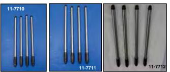
V-Thunder Evolution Pushrod Sets are made from .049 wall 4130 chromoly steel. Exacting tolerances for reliability. VT No. 11-7712 is a 2-piece style which can be removed or installed without disassembling heads. These rods fit stock or Velva Touch Tappet units. \*Note: Saves time without the disassembling of the heads or tappet blocks
