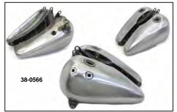
Fat Bob 3.5 Flatside Bobbed Tank Set features handshift gate provisions to fit early style gates for 1936-46. These flat side tanks feature screw type bungs. Order caps separately. Petcock fitting should be masked or plugged during painting for easy installation. The side tank features side shift tank mounts. For use with catege 1936-1946 type shifter gates or the conversion gate for 5 and 6 speed models, smooth type. VT No. 38-0566
