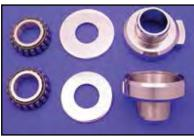
Chrome Big Twin Neck Cup Kit features built in fork stop on lower cup to accept 1988-99 FXST lower fork stem with integral stop. Kit includes chrome upper and lower cups with races, bearings and dust shields.
