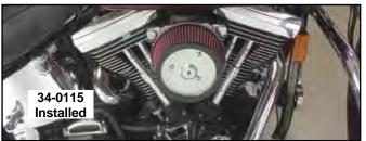
TC-88 Filter Upgrade Kit includes washable filter and longer stud set to replace Screamin' Eagle elements. There is 20% more air flow with this filter. Order cover separately. VT No. Item
