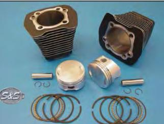
**Big Twin 3%**" **Big Bore Cylinder Kits** by S&S are supplied with fitted forged flat top pistons, ring, wrist pins, head and base gaskets. Stock crankcases must be machined to accommodate the larger spigot diameter. Available with black or natural finish cylinders. Fit 1984-99 Evolution.
