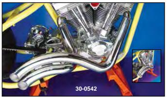
Before Starting Engine wipe all fingerprints off exhaust pipes after installation. Oil from hands will leave permanent marks on chrome finish.
