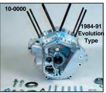
**S&S Crankcase Sets** are shipped set up with Timken left side bearing and race assembly, seal and seal spacer, oil pump drive bushing, needle bearing and pinion race for right side, (pressed in and line honed) ready to assemble. Also included are cylinder studs, nickel plated case bolts, crankcase fittings and a timing and magnetic drain plug. Accepts wheels up to 8½" diameter. Note: Oil pump required for assembly.
