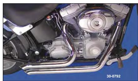
**Radii Exhaust Sets** feature "Quad Finishing" which includes triple dura nickel and chrome as the final finish. After chrome plating, pipes are normalized and dried @572° F for the final finish process.
