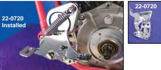
**Rocker Type Clutch Pedal Assembly**.Replaces 36810-65A for 1936-78 Big Twins. When installed on any 1965-78 FL, 18-3606, clutch release arm must be used. Order appropriate rod separately. For 1965-up primary applications order VT No. 21-0313 alloy spacer block separately.
