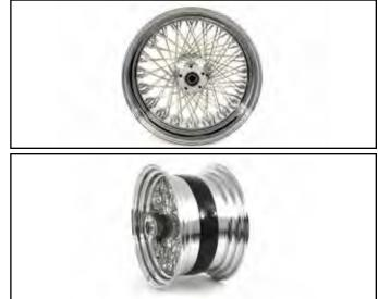
Wheel Assemblies with chrome billet hub for Softail models feature a chrome plated billet hub, chrome spokes and chrome steel rim for either tube type or tubeless application. Rear wheels have extension on pulley side to minimize pulley spacers and bearing is moved outboard to prevent bent axles. Front or rear wheels accept 111/2" disc rotors. Single flange are for right side drive. The 1984-99 hub types use Timken bearings and the 2000-up hub types use sealed bearings without ABS.
