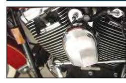
Chrome Head and Spark Plug Cover fits 1986-99 Evolution models. Covers are held in place by rubber inserts supplied. VT No. 42-0929
