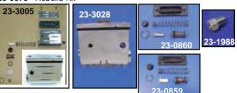
Chrome Rear Master Cylinder Assembly. Billet assembly is available in 5%" or 3/4" bore sizes. Features 21/4" spacing between mounting bolts, 1/8" NPT brake line fitting, milled body design and measures 31/2" long x 11/4" wide and 3" tall. VT No. Size 23-3028 5%" Complete Assembly 23-3005 ¾" Complete Assembly 23-0860 5/8" Rebuild Kit 23-0859 3/4" Rebuild Kit 23-1988 Fitting
