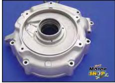
Motor Shop Alternator Sealing Ring Replacement Service. Ship in 1970-up left hand case with damaged O-Ring lip and we will machine out and replace with new steel sealing ring. VT No. 60-0164
