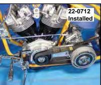
Police Style Jockey Shift Kit clamps to all Big Twin front frame with 11/8" tubes for 4-Speed ratchet type, 4-Speed rotary and 5-Speed model. VT No. 22-0711 and 22-0712 feature a smooth gate for shifting. Use either rocker clutch pedal or jockey pedal will fit with 3.5 or 5 gallon tanks.
