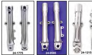
Chrome Lower Fork Slider Sets replace stock polished sliders on stock 41mm fork assemblies.
