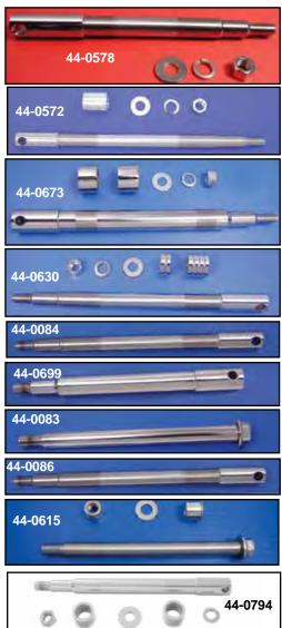
Chrome Front Axle Kits include plated axle, nuts, spacer, and hardware.
