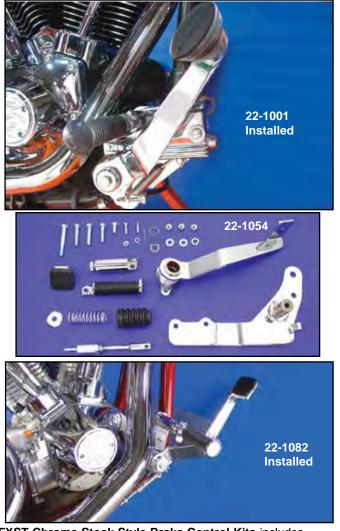
FXST Chrome Stock Style Brake Control Kits includes mounting bracket, lever and linkage. The 1982-86 type uses two bolt master cylinder. 1987-89 type has tab with square hole that uses spark plug. The 1990-up type fits models with frame mounted master cylinder. Master cylinder not included. VT No. Fits
