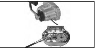
**E-Z Pull Clutch Assist** reduces manual effort required to pull the clutch lever by 40%. Mechanism fits inside transmission side cover and extends clutch operating mechanism for improved leverage.
