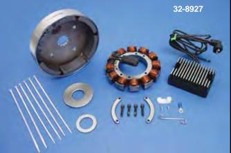
Big Twin Alternator Charging System features all components including stator, rotor, black solid state regulator, plug retainer and mount kit.
