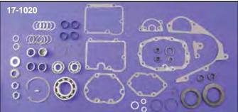
**5-Speed Jims Hardware and Rebuild Kit** includes bushings, locks, keys and snap rings for completing as 5 speed transmission rebuild. James gasket set included.
