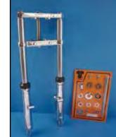
FXST Style Single Disc Fork Assembly features chrome trees with 1" stem, polished or chromed lower slider legs, to accept 11.5" caliper and brake disc, hard chrome fork tubes, axle, neck bearings, top cone and stem nut, pinch bolts and bearing dust covers. Fork is 31" overall length (L) and legs are assembled. Single disc unit accepts 11.5" brake disc and left side caliper. Voar
