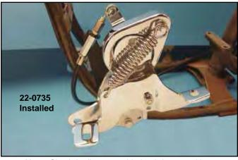
Note: Clutch is disengaged in heel down position.
