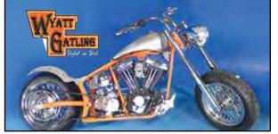
**1991-99 Softail Wide Right Side Drive Swingarm** in conjunction with parts listed allows use of 280-300 rear tire with a 1.5" belt. Swing arm is 2" longer than stock Softail tail section includes adjuster and 1" axle.
