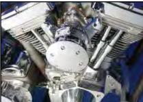
Velo-dome™ is Wyatt's velocity stack with built in cover for Super "E".
