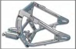
**Chrome Rear Swingarm and Shock Assembly** fits Softail models. Includes chrome tail section, adjustable shocks with 1" lowering capability, chrome axis tube with tapered allen screws and chrome shock mount bolts.
