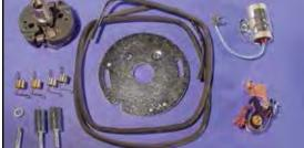
*Blue Streak* Sifton "Tuneable" Ignition Advance Assembly includes stainless advance base, points plate with "Blue Streak" points and condenser with hardware and 3 pairs of color coated springs which allow full advance at 1400, 2000 and 2600 RPM depending on which spring is selected.
