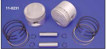
V-Twin Piston Kits include 2 cast alloy pistons, genuine Hastings 3-piece ring set, 2 wrist pins and 4 circlips. OHV Piston Set use 22588-78 pin lock, VT No. 12-0929 Standard Comp
