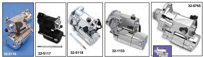
**High Torque Starter Motors** by Volt Tech are available in back or polished/chrome finish and in either 1.4 kw field wound or 1.7 kw permanent magnet types. Stock starter motor is 1.2 kw field wound type. Polished/chrome units have all aluminum parts polished and all steel parts are chrome plated. Black units are black powder coated.
