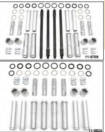
**Performance Pushrod Sets for TC-88** are E-Z install type which are designed to be installed without removal of the heads or rocker boxes. Rods feature chromoly tube construction with rolled thread adjusters. Fits 1999-up FXST-FLST-FXD and 1999-16 FLT.
