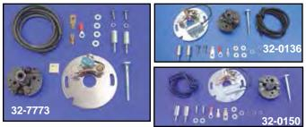
**Points Conversion Kit.** Both brands include everything necessary for direct replacement on 1970-78 Big Twin, 1971-78 Sportsters or for converting late model electronic-type back to points. Accel type available with microchip points, which will require a domed shaped points cover such as VT No. 42-0299 to accommodate taller points. The V-Twin unit includes stock style points and condenser. 32-0150 available with needle bearing weights.
