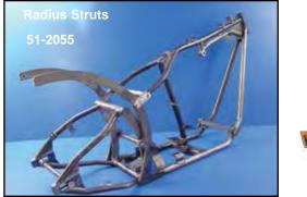
Wyatt Gatling Customizer Wide Drive FXST Frame manufactured from 1¼" diameter tubing with a 34° neck rake, 2" stretch in downtubes and 1½" stretch in backbone. Frame accepts a 200 series tire with belt by use of ½" offset kit, FXST oil tank and FXST flatside gas tanks. Frames include rear swingarm, radius style fender struts for 9" fender, front oil tank mount and rear axle.
