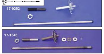
**5-Speed Clutch Push Rod Kits** are three piece. Replaces OE parts for all 5-speed transmissions.
