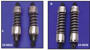
**Progressive Suspension 412 Series Chrome Shocks** are manufactured from the finest material available. Magnum 412 Series shocks are nitrogen charged with six-stage automatic damping and an adjustable spring preload. Available with chrome spring and end caps, shock cartridge is not chrome. All shocks are measured eyelet to center of eyelet.
