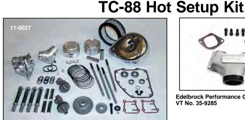
S&S TC-88 Cam, Carburetor, Pushrod and Piston Hot Setup Kit include Super "E" carburetor, adjustable pushrod set, pushrod covers, 570G cam (.570 lift), cam gear drive set and gear cover gasket kit. Installation of kit requires stock bore cylinders to be bored out to 3 7/8" and will increase compression ratio to 9.7:1 with stock cylinder heads. Order piston kit separately. VT No. 11-0027
