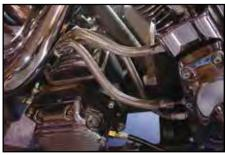
Custom Stainless Steel Oil Line Kit fits TC-88 for custom applications. Includes three compression fittings and three seal ends. Hose must be cut for installation. VT No. 40-0467
