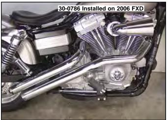
Sweeper Exhaust fits FXD models including 2006-up models with oxygen sensors. Pipes are 1<sup>3</sup>/<sub>4</sub>" to 2<sup>1</sup>/<sub>4</sub>" at end portion. Bracket included. Order baffle separately
