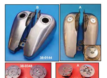
Air Craft Cap Style Bobbed Gas Tank Sets fit 1984-99 FXST-FLST or other flat side tank mount systems. Updated shape is tapered from front to rear. Filler neck available as "Bolt In" with insert held in place by 6 chrome allen screws or "Weld In" where insert is welded in place. Order appropriate caps separately.
