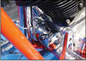
40-0315 Installed Oil Filter Adapter installed in the generator position. VT No. 40-0315
