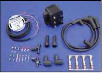
Daytona Twin Tec Internal Ignition Kit for 1984-99 Evolution Big Twin, 1970-84 Shovelhead Big Twin and 1971-97 Sportster models. Kit includes ignition, coil and spark plug wire set. VT No. 32-3015
