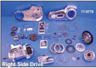
**1986-99 Softail 6-Speed Conversion Kit** includes complete assembled 6 Speed transmission with chrome mount plate, chrome top and chrome end cover, chrome inner and outer primary covers, full clutch pak and 1.7 kw chrome and polished starter with shaft assembly. Right Side Drive kits include hydraulic clutch side cover. Transmission accepts electric speedometer sensor (not included). **Right Side Drive Left Side Drive Case**
