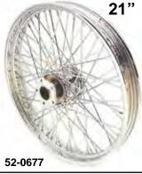
Complete 60 Spoke Wheel features chrome wide steel rim, steel hub and chrome spokes for any wide frame application. Hub features a .900" extension to minimize pulley spacers and the bearing is moved outboard to prevent bent axles. Accepts 11 1/2" disc rotor, 1984-99 style pulley or 1973-85 chain sprockets. Steel hubs include bearings, seals and spacers. Rim is sealed after truing so that it can also be used with tubeless tires.
