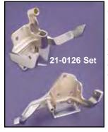
Chrome Brake and ShifterMount Plates replace original<br/>units on FLST models.VT No.OEMSideYears23-009542431-00Right00-0621-012233630-00Left00-0621-0126—Set00-06
