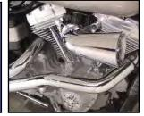
Turbo Funnel will mount on CV carburetor bolt pattern in a forward horizontal position. Order adapter plate 34-0693 to place in upright vertical position. Fits 1993-2007 Big Twin CV-Delphi-EFI VT No. 34-1197
