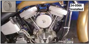
7" Evolution Type Air Cleaners include cover, foam, backing plate. Order brackets separately.
