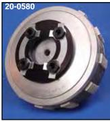
Pro-Clutch by Rivera Engineering converts old style clutch packs to smooth modern diaphragm spring function. Available for early chain or belt drive with wet or dry clutch. Kit includes clutch hub with bearing, clutch discs (friction and steel), diaphragm spring, spring retainer, pressure plate and four shoulder bolts. 1984-up kits utilize existing clutch basket, supplies a clutch hub to allow use of clutch plates that increase surface area by 100% to reduce slipping.
