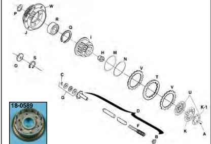
**1998-up Big Twin Clutch Parts.** Clutch Drum "J" has "W" Ring Gear installed.
