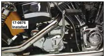
5-Speed Kick Starter Kit features slim profile design. Pushrod modification may be required. Order kick starter arm and pedal separately. Fits all 5-Speed replacement OEM transmissions.
