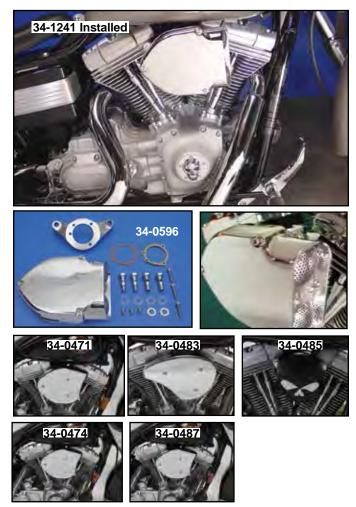
V-Charger<sup>™</sup> Chrome Air Cleaner for Big Twin features air scoop "blower" design and includes a built-in chrome screen and filter element. Kits include brackets and/or integral bracket, breather system except where noted.
