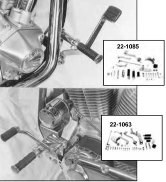
**FXST Chrome Replacement Style Forward Control Kits** include mounting brackets, levers and correct linkage for 1982-99 FXWG and FXST models. Master cylinder not included.
