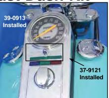
FLH-FXST Dash Kit features chrome cast dash with lens and hardware, 6-post switch, choke cable and knob, all mounting hardware and trim strips. Stock on 1968-84 FLH- FXWG, 1984-95 FXST-FXWG is 2240:60 ratio. Can be adapted to all 3<sup>1</sup>/<sub>2</sub> and 5 gallon tanks. Dash base has wiring and sockets. Spacer kit VT No. 39-0209 is included to mount on 1984-99 Flat side tanks. Choose the proper cable for each application.
