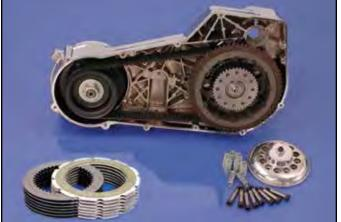
**BDL 8mm x 42mm Electric Start Belt Drives.** Includes a polished pressure plate, Kevlar clutch, sealed inner primary bearing and features a shorter length clutch hub that eliminates unnecessary weight past the end of the mainshaft and can be installed without any modifications to inner primary.
