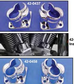
**Chrome Evolution Tappet Covers** fit over stock blocks. Each cover has a slot which allows it to be installed without removing pushrods. Install by lifting the pushrod tube cover and inserting the covers. Fits 1985-99 Big Twins.
