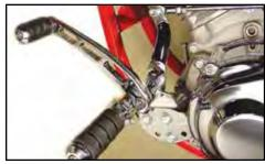
Chrome Billet Shifter Lever features slotted design. Fits 1990up FXST and 1991-up FXDWG. VT No. 21-0670
