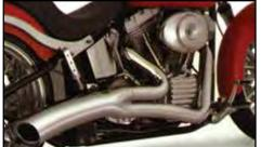
Chrome Vance and Hines Big Radius 2 into 1 Header breaks the mold. Fits 1986-2010 FXST. VT No. 30-1586
