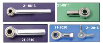
Self-Aligning Rod Ends. Heim joint type swivel allows alignment up to 28° off center. Self lubricating brass ball socket available for shifter or brake rod ends, 5/16 x 24 or with 5/16 hole. 21-2016 has 5/16 x 24 stud.
