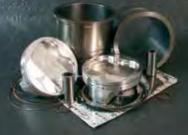
**1320cc Big Bore Kit** for V-Rod includes 12:1 compression forged Wiseco Piston Set with rings and matched 4.250 bore gaskets and sleeve set. Case boring required.
