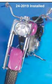
FLST Style Complete Front End Assembly includes the complete fork kit with the addition of the five piece chrome fork cover set, 7" headlamp and bracket, 16" chrome wheel, speedometer drive, chrome caliper, 11.5" drilled disc and fat kid style or FLST style fender.
