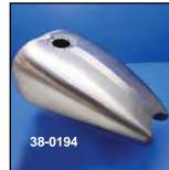
Smooth One-Piece Tanks fit 1984-99 Softail models are 4.2 gallon, stretched and includes hardware for mounting. Order stock bung caps separately. Some seats may not match up. VT No. 38-0155 is a 2" stretch 1 piece tank with a 2" extension welded on. 38-0273 does not have seat cut out.
