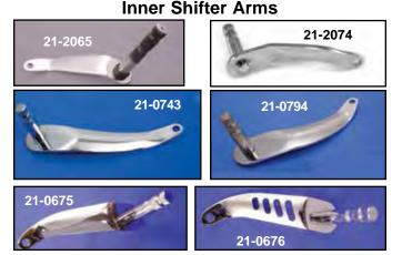
Chrome Inner Shifter Arms fit through frame mount shifter plates on Big Twins and feature splined ends.
