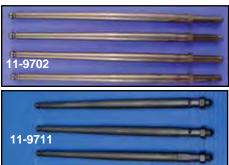
**Tapered Adjustable Pushrods** are manufactured from 4130 steel with hardened adjusters and ball ends. Designed to be installed without removing gas tank, rocker box or camshaft cover. Set of four. Fits Evolution Big Twin hydraulic or solid.
