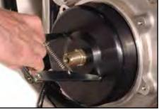
Big Twin Alternator Rotor Puller uses the two threaded holes in rotor to allow removal of rotor. VT No. 16-0693
