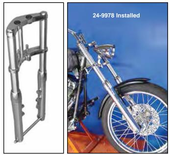
**Chrome Billet Style Fork Assembly** features chrome machined triple tree set with "hidden" top nut. Chrome leg assembly is smooth style to accept 2000-up left side caliper and a FXSTD style fender. One inch neck bearing and axle kit included.
