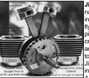
Jims 116" Stroker Kits with natural finish cylinders. Each kit includes a balanced and trued flywheel assembly with integral pinion shaft, sprocket shaft and crank pin for maximum stability and resistance to flywheel distortion. Each kit is press fit with Jims H-Beam forged connecting rods and prebalanced with Arias pistons. Fits all 1999-06 carbureted Twin Cam A motors only. 45%" stroke and a 4" bore. VT No. 11-2053
