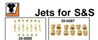
Jet Assortment for S&S Super 'E', 'G' and 'B' carburetors. Complete kit includes 7 intermediate jets from .025" to .033" and a main jet kit only which includes 14 main jets from .062" to .084".
