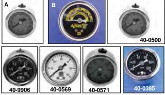
Liquid Filled 11/2" Oil Pressure Gauges feature a weather resistant sealed lens, stainless steel case, chrome rim and extra heavy mechanism. The liquid filled face eliminates needle bounce giving a constant reading. All gauges have 1/8" NPT male rear fitting.
