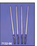
**Crane Adjustable Pushrods** made from aircraft grade seamless 4130 chromoly steel tubing and heat treated to 128,000 psi tensile strength for a stronger and lighter than stock pushrod. New style adjuster helps minimize the effects of poor geometry found in stock pushrods, the smaller diameter eliminates pushrod "rub" completely. Set contains two intake and exhaust pushrods. These are not the time saver type.
