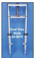
FXWG 10" Style Dual Disc Fork Assembly fits 1982-94 FXR and is available with polished or chrome lower sliders which are smooth at the reflector boss area, accepts dual disc calipers, 10" brake disc, chrome trees, bearings, axle, spacer and top nut. Hard chrome tubes with internals are assembled. Stock is 31" overall length. Units do not include provision for fork lock
