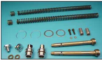
Fork Tube Assemblies include chrome fork tube plug and caps, seals, springs and damper kit. Fits 1984-99 FXST. VT No. 24-0742
