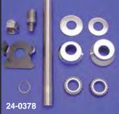
Raked Neck Kits include chrome cups, bearings, dust cover, stop tab and longer stem. Longer fork tubes required for installation. Fit 1991-05 FXD. VT No. Rake 24-0378 3° 24-1286 5°
