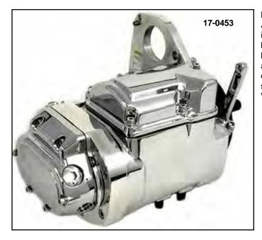
Motor Shop Ready 6-Speed FXST Polished Transmission Assembly for 1991-99 models. Features include either polished case, chrome top and side cover, machined shift forks, heavy duty trap door, precision ground full width gears with back cut dogs and pulley. Each unit is completely factory assembled to OEM specs. Unit is close ratio 1st gear 2.94:1 overdrive 6th gear .86 :1. Accepts 1996-up speedometer sensor VT No. 17-0561. VT No. 17-0453
