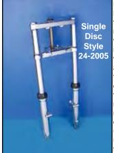
FXST 11.5" Single Disc Style Fork Assembly fits FXR 1982-94 or 1991-up FXD Dynaglide models. Assembly is available with chrome triple trees, polished or chrome lower legs without reflector boss to accept a left side single disc 1984-99 type caliper and 111/2" brake disc. Hard chrome fork tubes with internals assembled, axle, neck bearings, top cone, stem nut, pinch bolts and bearing dust covers are included. Stock unit is 31" overall length. FXR units do not include provision for fork lock.
