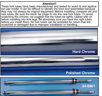
41MM Fork Tube Assemblies are hard chrome finish. Include top plug, springs, spacers and internal pieces completely assembled. Order bushing set separately, 1984-99 FXST,1984-96 FLT, 1986-99 FLST, 1993-99
