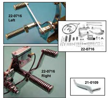
**Chrome Forward Control Kit** fits 1958-86 Big Twins, 1986-99 FXST. Includes shift and brake sides including <sup>3</sup>/<sub>4</sub>" bore chrome Kelsey Hayes style master cylinder. Kit is supplied with O-ring pegs, but can be replaced with other style of clevis mount pegs. A universal nylon brake line kit, chrome mount hardware and 4 and 5 speed styles shift rods are also included.
