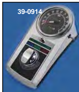
FLH Dash Kit features chrome cast dash with lens and hardware, 6-post switch, choke cable and knob, all mounting hardware and trim strips. Stock on 1968-84 FLH. Can be adapted to all 3.5 or 5.0 gallon tanks. Dash base has wiring and sockets. Choose the proper speedometer cable for each application.
