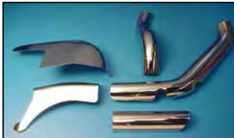
1970-84 FLH Heat Shield Set includes 5 pieces, 2 for the left and 3 for the right side to fit dual cross over systems. VT No. 30-0350
