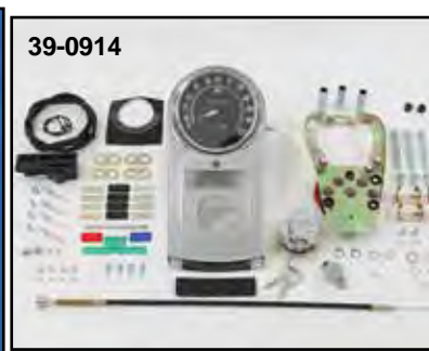
FLH Dash Kit features chrome cast dash with lens and hardware, 6-post switch, choke cable and knob, all mounting hardware and trim strips. Stock on 1968-84 FLH. Can be adapted to all 3.5 or 5.0 gallon tanks. Dash base has wiring and sockets. Choose the proper speedometer cable for each application.
