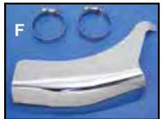
Chrome Heat Shields fit 1970-84 FLH models, not FLT. Worm clamps included.
