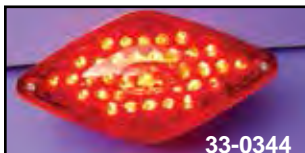
Diamond Rear Lamp features a red lens, 12 volt, bolts to stock FXWG-FXST or to cateye mount holes.
