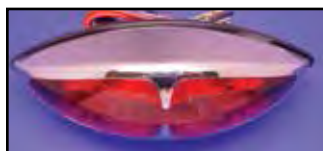
Chrome Big Eye Tail Lamp are constructed of ABS. VT No. Lens Type 33-0643 Clear LED 33-0644 Red Bulb
