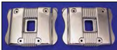
Chrome Lower Rocker Box and Gasket Set fits 1991-03 models. VT No. Item 42-0220 Kit, 1991-03 43-0165 Lower Only 1999-03
