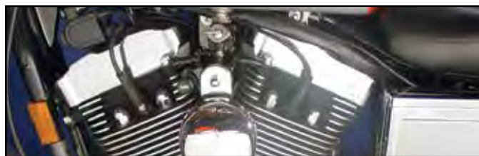
Chrome Rocker Box Dress Cover Sets fits over rocker box assembly without dis- assembly of engine. Chrome allen screws included. Fits 1986-up. VT No. 42-0796
